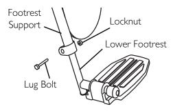
FIGURE 6.3 Footrest Height Adjustment
